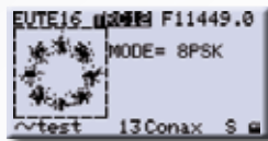
Costell. DVB-S2 = 8PSK, T = COFDM, C = QAM & modulation parameters
